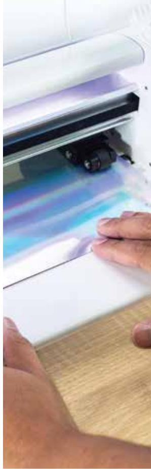
Thanks to adjustable pinch rollers, you're not limited to a specific cut area. Utilize the entire width of the cutter for your projects - and you can choose whether or not to use a cutting mat!
