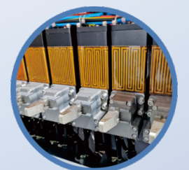
Build-in heaters & Negative pressure
